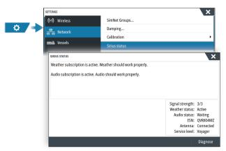
The status panel shows signal strength is indicated as 1/3 (weak), 2/3 (good) or 3/3 (preferred). It also includes antenna status, service level, and the electronic serial number for the weather module.
