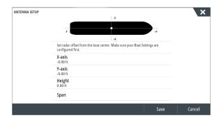
The approximate position of the antenna on the vessel must be set in order to correctly position the vessel outline when viewing close range settings. The PPI will be centered on the icon representing the position of the antenna.
