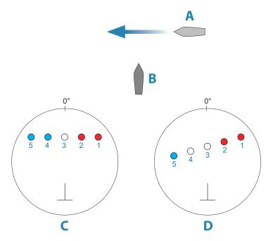
The examples show the target movement (1-5) over 5 radar scans with the radar in relative motion mode.
