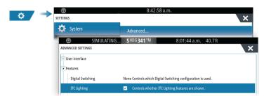
Once the ITC lighting controller is installed and connected to the NMEA 2000® network, it should appear in the control bar. If it is not appearing in the control bar, you can activate it from the Advanced settings dialog.
