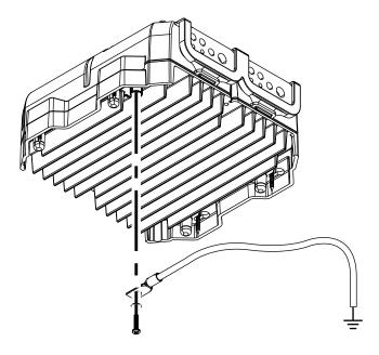
Alternatively, you can ground the RI-50 using the **CASE / SHIP GND** spade terminal on the circuit board.
