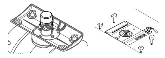
2 On the antenna, check the sealing ring is correctly positioned in the groove around the waveguide.
