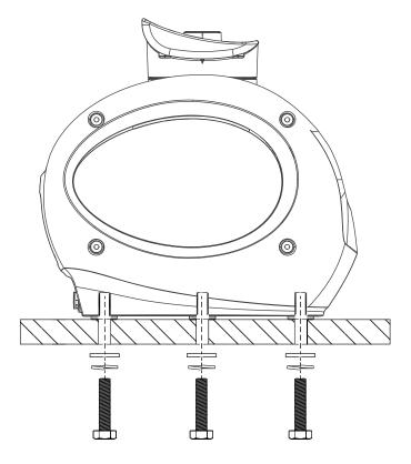
If you are installing the pedestal onto a steel surface, also use the supplied plastic isolating washers.
