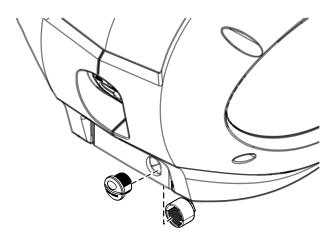
4 Re-route the connector to the bracket and secure it with the retaining nut.
