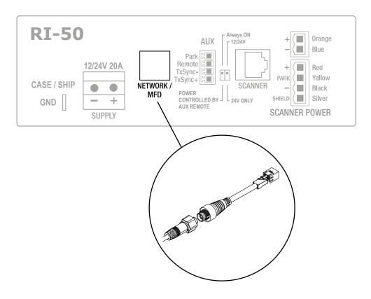
The RI-50 can be connected directly to any Simrad®-compatible multi-function display or to a network switch such as an NEP-2.
