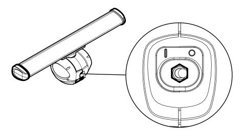
4 Disconnect the interconnection cable from the pedestal.
