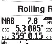
A single page displaying: current waypoint name, distance to waypoint, course over the ground (COG), speed over the ground (SOG), bearing to waypoint, cross track error and turn angle. A rolling road diagram illustrates the vessels course in relation to the direct track from the previous to the current waypoint and the direction to steer to return to the direct track.
