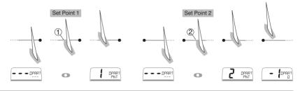
The line for Depart calculations is between the positions you set. Set your points as close to the ends of the actual start line as possible.
