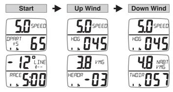
Programming these pages into the Autoleg Page prior to the race would automatically show these pages for the appropriate leg of the course; leaving the tactician free to concentrate on the race, not on configuring his instruments.
