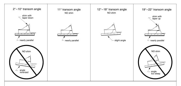
Figure 11. Sensor angle adjustment
