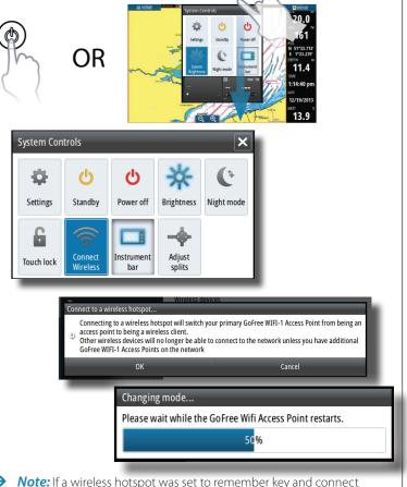
*Note:* If a wireless hotspot was set to remember key and connect automatically and is in range. The WIFI-1 will connect to it automatically
