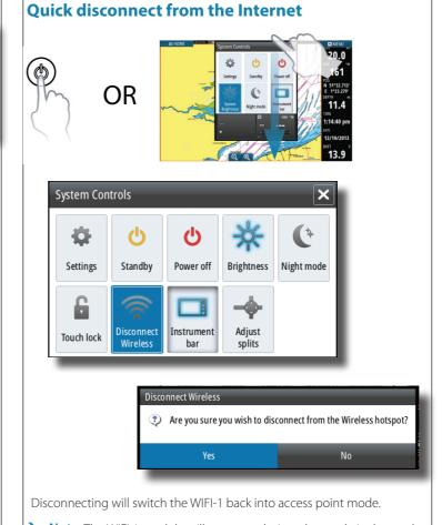
→ Note: The WIFI-1 module will restart each time the mode is changed. The WIFI-1 will be off line for up to two minutes.
