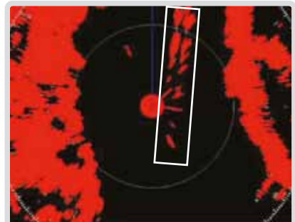
Poles and vessel are less defined on pulse radar display.
