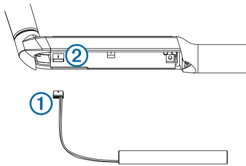
The connector fits into the port only one way. Forcing the connector into the port may damage it.
