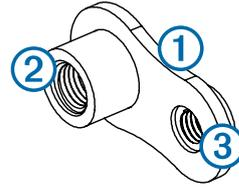
The smaller 3.5 mm ( $1/8$  in.) hole ③ on the nut plate should line up with the smaller hole on the template.
