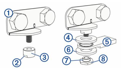
**NOTE:** If there is adequate clearance for you to tighten the bolts after the linkage is assembled, you may find it easier to secure the bracket to the kicker motor tiller arm after you have assembled the linkage on the bracket.
