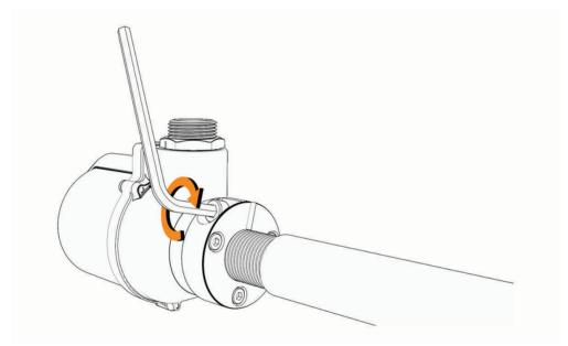
6 Slide the seal onto the other end of the steering actuator, and rotate it clockwise to attach it to the tilt tube.
