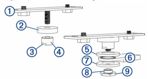
**NOTE:** If there is adequate clearance beneath the motor for you to tighten the bolts after the linkage is assembled, you may find it easier to secure the bracket to the kicker motor tiller arm after you have assembled the linkage.
