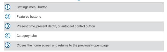
The categories tabs provide quick access to the main features of your chartplotter. For example, the Sonar tab displays the views and screens related to the sonar feature. You can save items you commonly access to the Pinned category.
