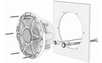
**18** Secure the speaker to the mounting surface using the included screws.
