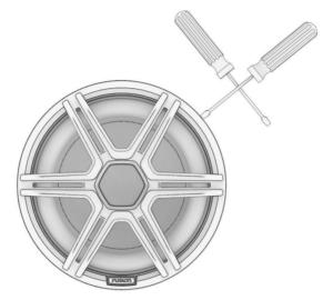
**NOTE:** For the best results, avoid placing the prying tool in the middle of a retention tab. The grille is easier to remove when starting at either edge of a retention tab.
