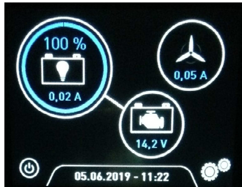
Figure 5 : Shunt #1 with additional battery (+2) and shunt #2 in Energy Mode
