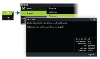
The status panel shows signal strength is indicated as 1/3 (weak), 2/3 (good) or 3/3 (preferred). It also includes antenna status, service level, and the electronic serial number for the weather module.
