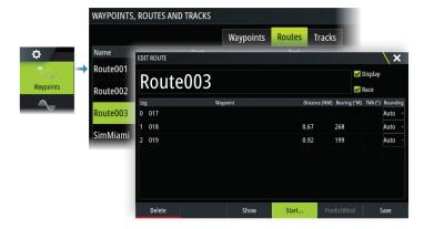
When route navigation is viewed, the menu expands and shows options for canceling the navigation, for skipping a waypoint, and for restarting the route from current vessel position.
