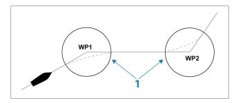
The arrival circle (1) should be adjusted according to boat speed. The higher the speed, the wider the circle.
