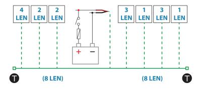
→ Note: Do not connect the NMEA 2000 power cable to the same terminals as the engine start batteries, autopilot computer, bow thruster or other high current devices.
