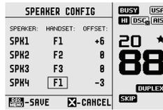
You can associate one or more External speakers to any Fixed handset. For each of the four External speakers select a Handset to be associated with it.
