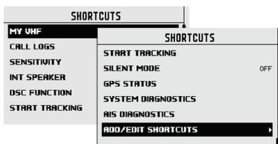
→ **Note:** The MY VHF page is available to the operator only when enabled as a shortcut – or by long pressing the **VOL/SQL** selector key.
