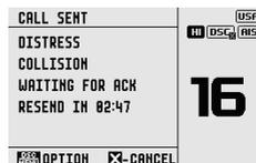
The Distress Call is automatically re-sent every 3.5 to 4.5 minutes until a distress acknowledgement (DISTRESS ACK) is received.
