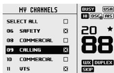
Subsequent opening of this page will show a list of only the selected channels. Choosing one of the channel options immediately exits the page and sets the radio to that channel.
