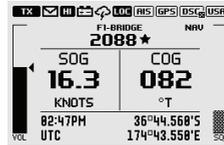
Press the **X / POWER** key to exit NAV mode and return to normal radio operation mode.
