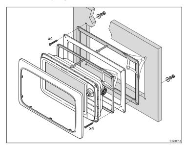
Peel off the protective layers of the adaptor gasket and affix to the back of the adaptor plate.
