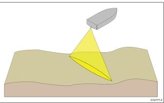
**DownVision**<sup>™</sup> is effective at lower vessel speeds. In deeper waters the CHIRP bandwidth is automatically optimized to improve bottom lock and the detection of moving objects (e.g. fish) in the wider water column.
