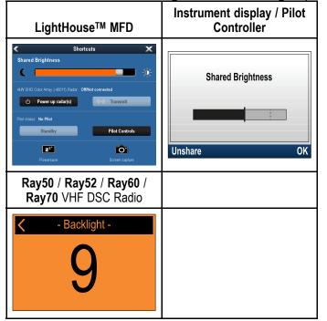
Multiple brightness groups can be configured. These groups could be used to reflect the physical location of units on your vessel. For example, the units at your helm can be set to one group, and the units on the flybridge can be set to a different group.
