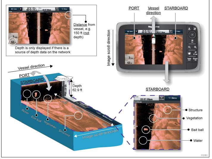
SideVision<sup>™</sup> images are constructed line-by-line, similar to the way a television picture is composed of many horizontal lines. Each successive ping from the SideVision<sup>™</sup> transducer adds a new line of image data to the top of your display. Each new line shows sonar returns from both the port and starboard sides of your vessel.
