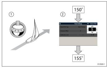
1. Set your vessel on a known heading and check the steering compass.
