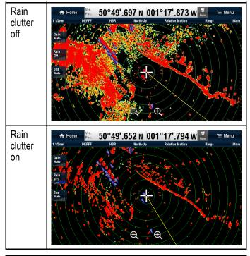
**Note:** Quantum uses pulse compression which filters out precipitation. However, you can identify/display precipitation using Quantum's **Weather** mode.
