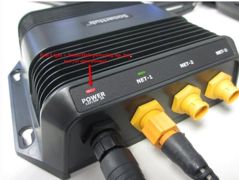
When the SonarHub is fully powered up and operational, the Power Light will be green.
