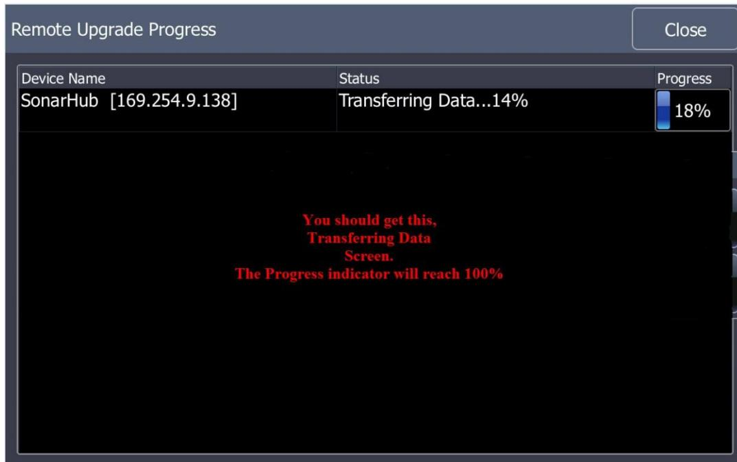
When the Data Transfer reaches 100%, Synchronizing File System will appear on the screen; this is the SonarHub upgrading the software and it will remain on this screen until the upgrade is complete.
