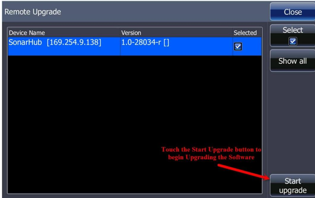
The unit will start Transferring Data from the SD card to the SonarHub.
