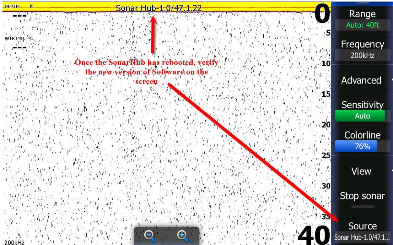
Please check the software version of the SonarHub once updating is completed. Updated version should read SonarHub-1.0-47.1.26-8.0.28295-r1. If the software version on the display matches the SonarHub has been successfully upgraded. You are now ready to disconnect the upgraded SonarHub and connect another SonarHub and repeat the process.
