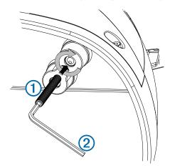
7 Install the isolators ③ over the threaded rods, and push them securely onto the four raised locations on the bottom of the pedestal ④.
