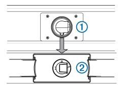
3 Secure the antenna to the pedestal using the included hex bolts (3) and spring washers (4).
