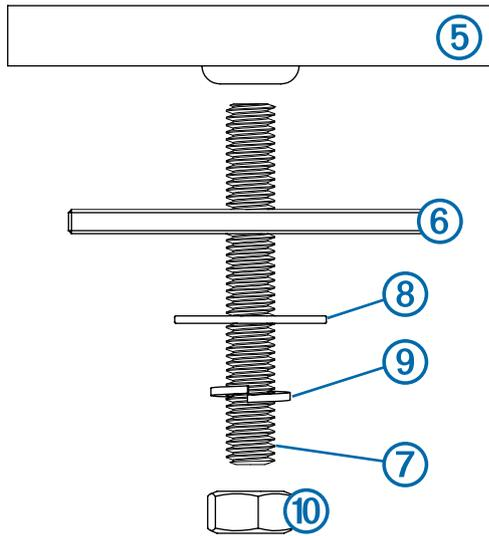
10 Using a torque wrench, tighten the nuts from 13.7 to 18.6 N·m (10 to 14 lbf-in.) of force.
