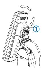
2 Tilt the device forward, and lift it out of the cradle.
