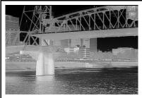
Thermal camera — provides night-time imagery, based on temperature differences between objects. Thermal imaging produces a clear image even in total darkness.
