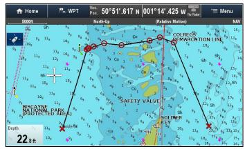
The generated route is based on the data available on compatible cartography compared with user defined settings. Waypoints automatically generated will be restricted from entering areas that do not adhere to the user defined settings.
