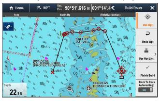
Waypoints within the route that were calculated using automatic route generation are assigned the Marker waypoint symbol.
