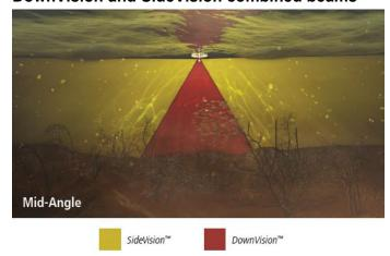
Note: When SideVision™ and DownVision™ systems are pinging simultaneously, some interference between the two systems may occur. To minimize interference between the systems, careful consideration must be given to transducer location. Raymarine recommends that you refer to your local dealer for installation advice.
